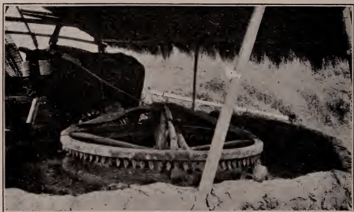
FIG. 141. - Close view of power wheel with cow attached, used in driving the irrigation pump, one of the two seen in Fig. 140.
