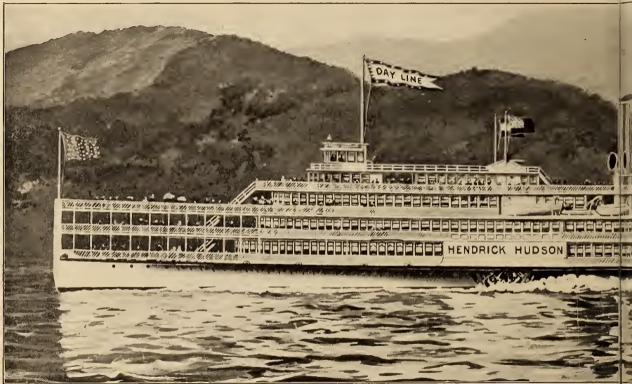
HUDSON RIVER DAY LINE STEAMER "HENDRICK HUDSON," the world's largest, most magnificent and swiftest river steamboat; built at a cost of $1,000,000; the main wheel-shaft is below deck, and there is no walking-beam, the 24-ft. paddle wheels being driven by a three-cylinder inclined compound engine, all the machinery being in the hull; the ship is a hotel, with numerous parlors exquisitely decorated. Designed by Frank E. Kirby, of Detroit, Mich., assisted by leading marine architects. The hull is built of steel.
