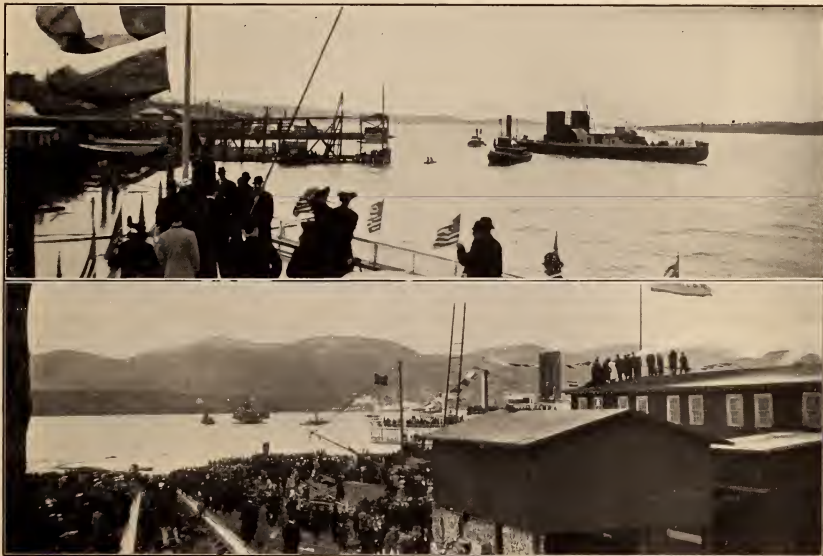
HUDSON DAY LINER "HENDRICK HUDSON" floating on even keel in Newburgh Bay after the launching, March 31, 1906. "HENDRICK HUDSON" seen from Marvel Shipyards after launching, a tug making fast to tow the hull down to W. & A. Fletcher Co.'s yards at Hoboken to receive magnificent superstructure and machinery, which are to be triumphs of the arts of joiner, decorator and engineer.
