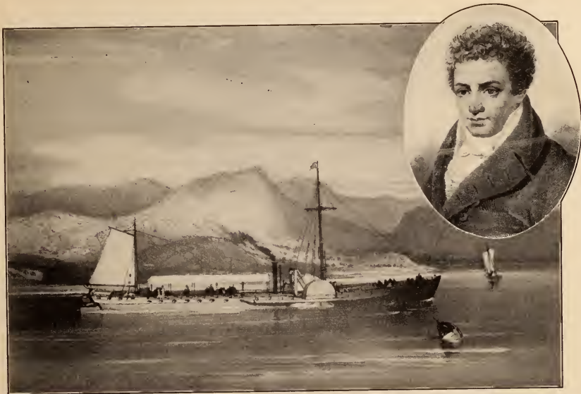
ROBERT FULTON and his STEAMER "CLERMONT," first successful steamboat; 133 ft. long, 16 ft. wide. Launched in spring of 1807 in East River, this primitive side-wheeler made its trial trip to Albany, August 7, and the following summer began regular trips between the metropolis and the state capital, thus inaugurating steam navigation. Fulton, after building other and faster boats, died suddenly in 1815.
